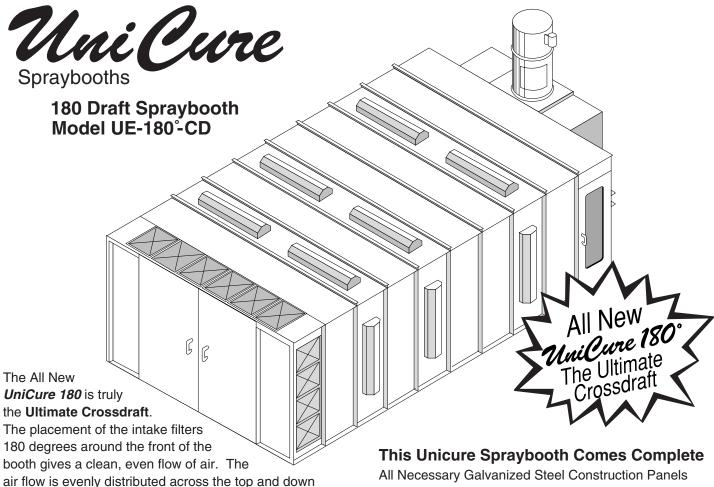
each side of the Vehicle. A 30" exhaust fan moves the required amount of air with very low noise level. The air is exhausted in the rear center area, 8 ft, wide and 7 ft. high which puts the finishing touch to the UniCure 180's ultimate air flow.
