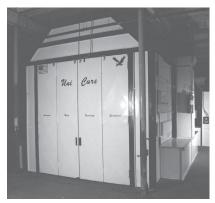
This booth is pre-fabricated, pre-fitted and holes are pre-punched from 18 gauge galvanized steel. The air is double filtered for the cleanest air possible. The intake air is pulled through the side filters then through the ceiling filters. The exhaust air is pulled out either side of the booth or through a floor pit. Efficient operation, clean air and a clean environment is what you get with this UniCure Truck Spraybooth.
